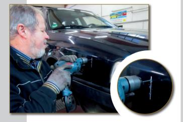
Increase the size of the middle hole to 25.7 mm. Using a step drill might help you. Enlarge the hole at the left and right side with a file so that the base and its 2 bolts will fit.
